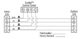
Figure 23: Low Voltage EcoNet™ Wiring
