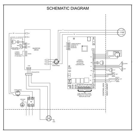
Figure 32: (-)A18AZ Wiring Diagram & Schematic Diagram
