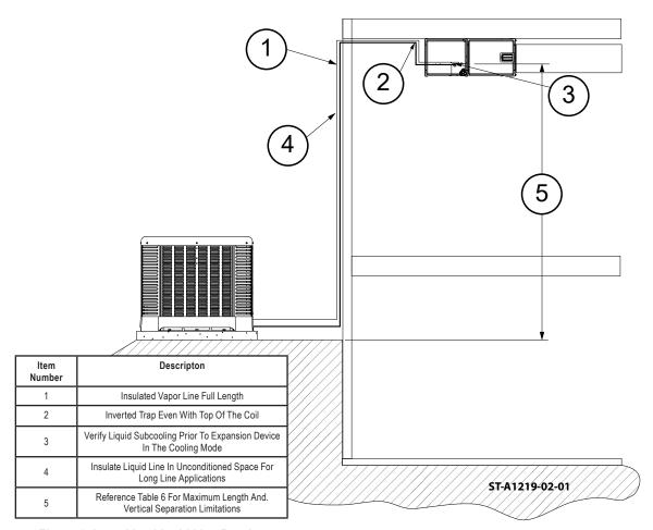
Figure 9: Long Line Liquid Line Routing
