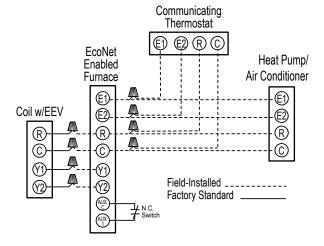
Figure 35: Thermostat Wiring for Heat Pump with Coil and Furnace
