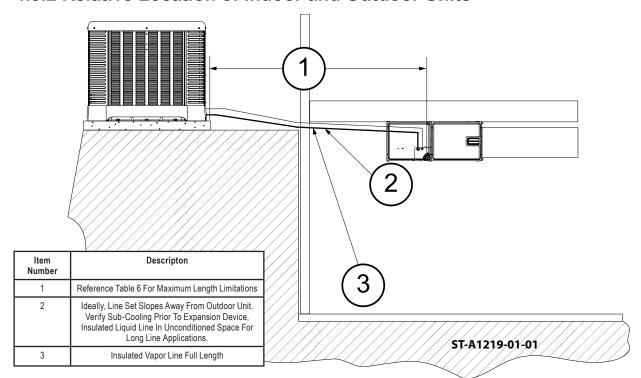
Figure 8: Slop Vapor Line Toward the Indoor Unit
