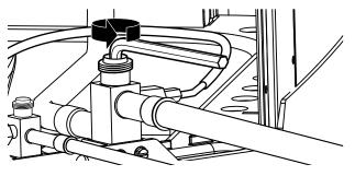
Figure 21: Open Both Service Valves
