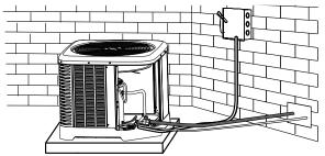
Figure 19: Insulate Vapor Line
