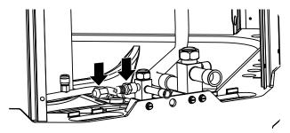
Figure 12: Remove Caps and Schrader Cores
