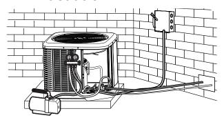
Figure 20: Evacuate Air and Moisture from System
