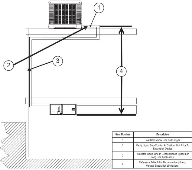
Figure 10: Liquid Line Routing for Unit Installed Above Indoor Coil
