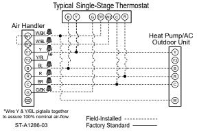
Figure 25: Typical Single-Stage Thermostat: Heat Pump With Air-Handler
