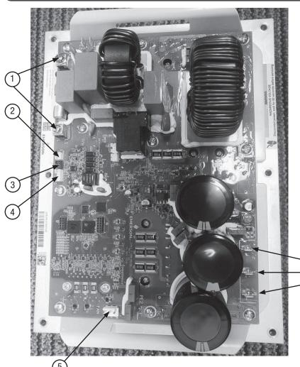
Table 13: Features on the Power Inverter Compressor Control
