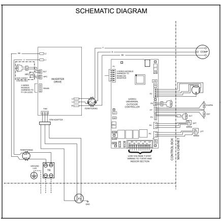
Figure 33: (-)P18AZ Wiring Diagram & Schematic Diagram
