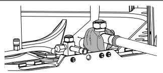
Figure 14: Wrap Valves Before Applying Heat
